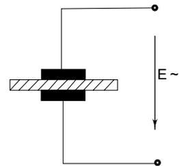
**Fig.6.3** Schematic electrode arrangement for testing dielectric strength
