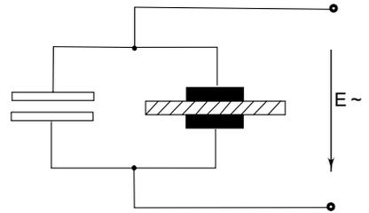
**Fig. 6.4** Electrode arrangement for testing dielectric constant
