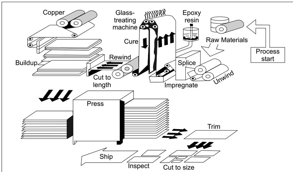
**Fig. 6.2** Process for manufacturing laminates (Courtesy GE Electromaterials, 2001)
