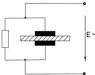
**Fig. 6.5** Electrode arrangement for testing dissipation factor
